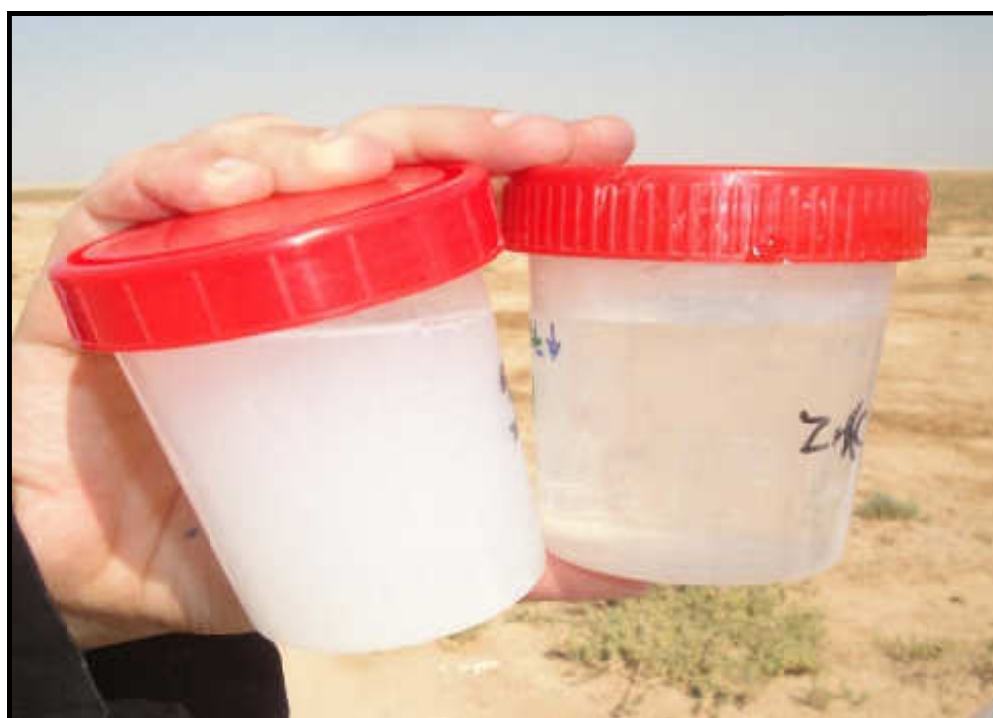
Figure 2-3: Foggy color solution at left due to H_2S gas fixation on-site in the field; sample on the right untreated chemically.
