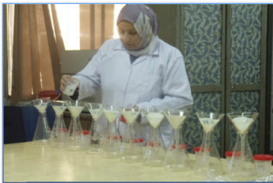
Figure 2-9: Filtration of the water samples and H_2S determination.
