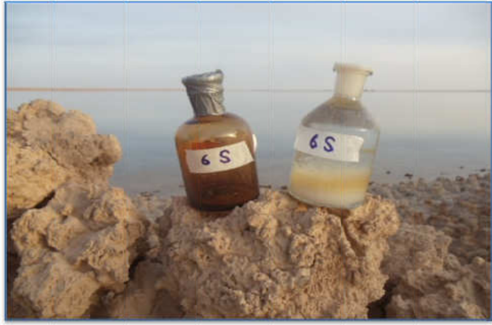
Figure 2-10: Water sample no. 6S for BOD measurement; Right bottle contains water sample with 2 mls of \text{MnSO}_4 as well as Azide \text{Na}_3\text{N} , whilst bottle on the left contain just the sample water.
