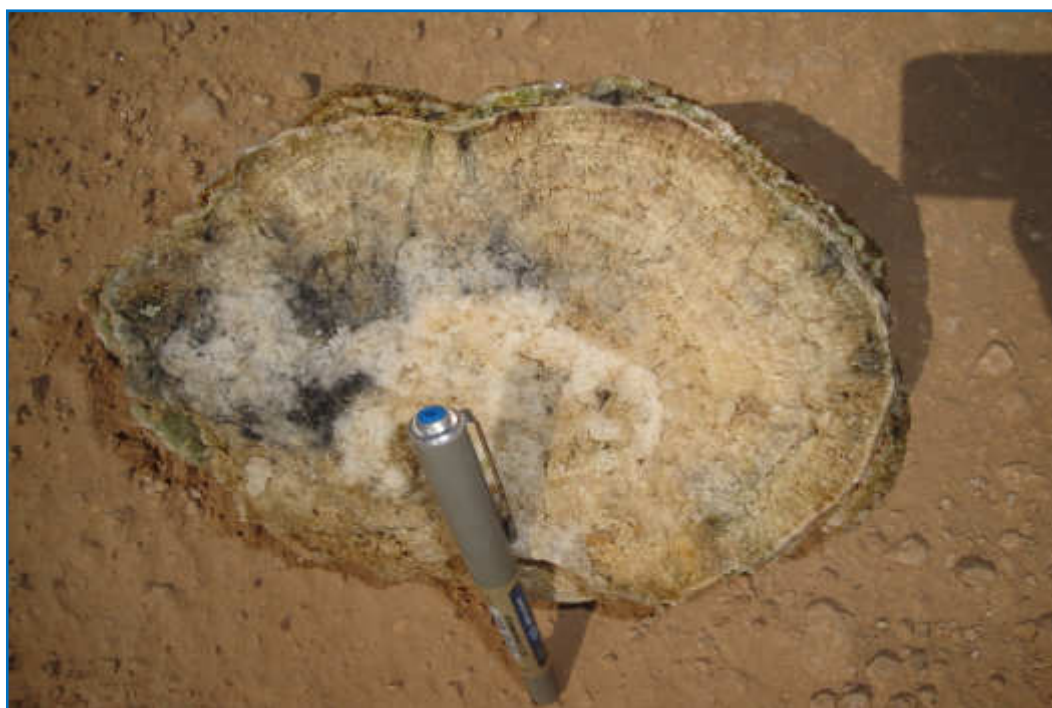
Figure 5-2: Cross section of gypsum mass show the internal structure as concentric circles; sample no. 11S-t.
